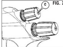
**WARNING:** When you reinsert the knob (6) on the adjustment (B) and before to tighten the countersunk socket screw (C), make sure that it is pushed in until it completely covers the face of the hexagon knob of the adjustment (Fig.2).
